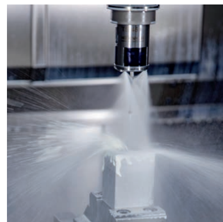
Cleaning with cooling lubricant
