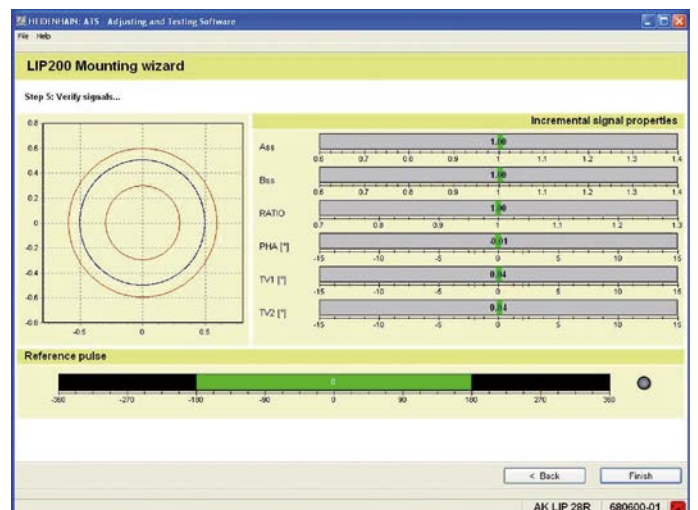
Commissioning using PWM 20 and ATS software
